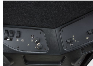
Switches Conveniently Located on Ceiling
