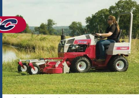
**Rear Discharge Advantage:** Cut materials are discharged to the back of the mower instead of your pond or flower bed.
