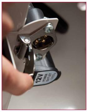
The Rear 12 Volt Power Outlets mount securely in the Ventrac 4000 series storage compartment. This keeps them out of sight and safe from moisture. Each outlet has its own spring-loaded cover for protection from any outside materials that may come into contact with storage box.
