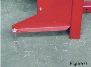
Insert the  $3/8 \times 4-1/2$ " bolt into the bottom of the main frame. (Figure 6) These act as legs for the spreader to set on when not in use.
