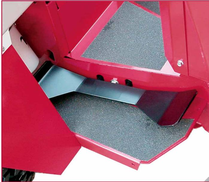
The optional Foot Control Pedal can free your right hand up for forward and reverse motion on the 4000 series. This is necessary for operating the VERSA-loader attachment and helpful when using the optional rear 3-Point Hitch.
