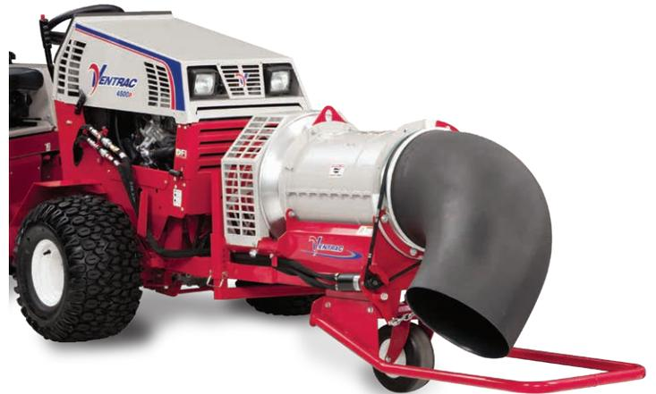
The Ventrac ET200 makes quick work of any clean up job. The Turbine Blower is designed to blow large volumes of air, and is much quieter than a conventional leaf blower. The ET200 can be used to blow leaves, light snow, and remove debris from sidewalks, parking lots and other areas.
