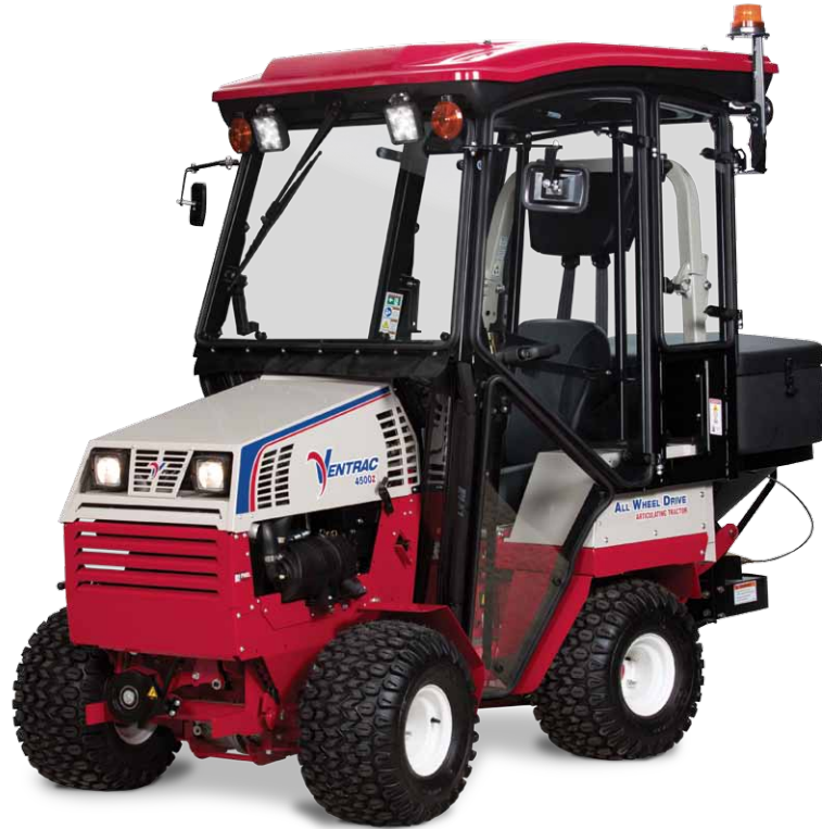
Cab shown with optional Directional/Hazards, Strobe Beacon, & Mirrors installed on a 4500Z with a SS575 Spreader.
