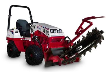
The KY400 Trencher is capable of trenching up to 40 inches (102cm) in depth with a 5½-inch (14cm) wide cut. It is designed with dual Push-N-Pull cylinders to assure positive boom control for digging, boom lift, and transport.
