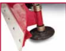
Hardened Cutting Edge and Skid Shoes
