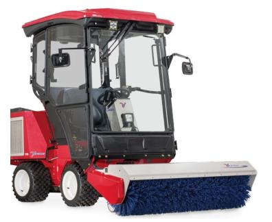
The LB540 Power Broom is designed for the sweeping and removal of snow, leaves, dirt, light gravel, and other materials from parking lots, sidewalks, and other surfaces. Heavy duty nylon bristles make short work of any clean up job without damaging the surface below
