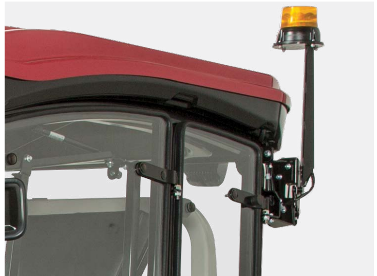
Fully Sealed, Breakaway Mounted Optional Strobe Beacon
