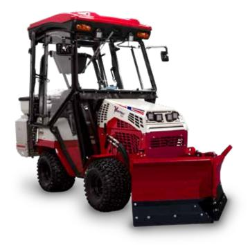
The 53.125-inch wide Ventrac SE530 V-Blade maximizes efficiency with the ability to quickly change from V-plow to scoop to straight blade, all from the convenience of Ventrac's exclusive S.D.L.A. Control System. With a 47.5" V width, the SE530 is ideal for walks and areas that larger blades are unable to plow.
